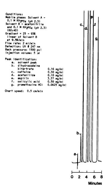
FIGURE 1. HPLC separation of standard solution on a  $\mu Bondapak$  C<sub>18</sub> column (dp = 10  $\mu$ m, 300 X 4 mm).
